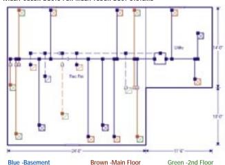
It's now easy to see several floors of ducts stacked on top of each other, and to be able to follow ducts to risers and then up or down to other floors. Ducts are the same color as the floor they're on. So blue ducts are in the basement, brown ducts on the first floor, green on the second, etc. Risers can be dragged to their correct interior wall location.
